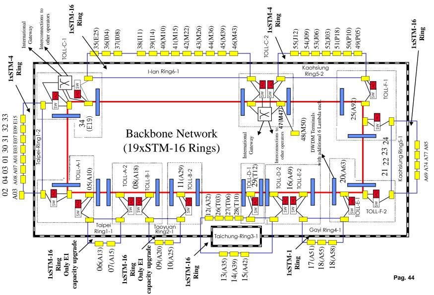
PHASE 4 Backbone and Region network structure for Switching and Internet traffic transmission
